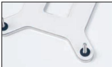
2. Place the LGA775 backplate under the motherboard aligning the screws to fit through the four holes available around the CPU as illustrated.
