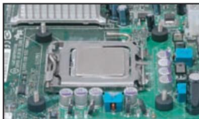
4. Apply the proper amount of thermal compound (part N) on the CPU surface; a thin layer is ideal, extra thermal compound will not improve performance. Make sure the CPU surface is perfectly clean.
