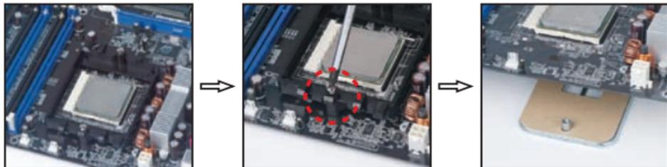
2. Place the backplate provided (Part E) below the motherboard aligning the two standoffs with the holes in the motherboard as illustrated.
