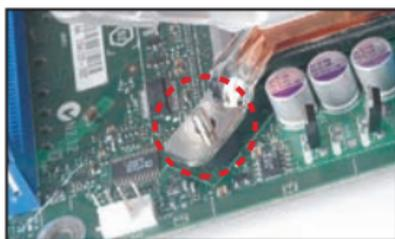
6. Secure the cooler with the collar nuts (part B), one for each screw, tighten the nuts gradually in a crosswise manner.
