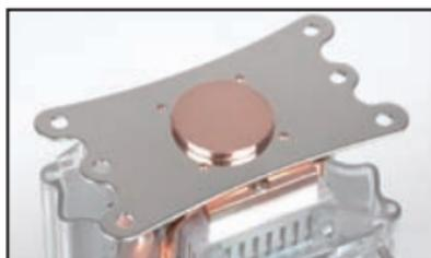
3. Secure the heatsink retention bracket with four (4) screws from step three.
