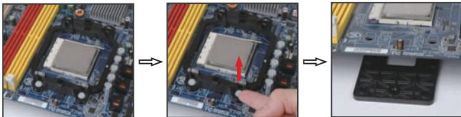
2. Place the backplate provided (Part F) below the motherboard aligning the four standoffs with the holes in the motherboard as illustrated.
