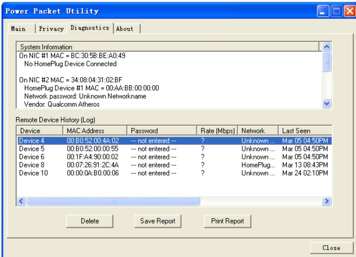
The **Lower panel** displays the history of all remote devices appeared on the computer over a certain period of time. All the devices and the parameters of the devices on the powerline network are listed. Devices that are active on the current logical network show a transfer rate in the rate column. Devices on other networks, or devices that no longer exist are shown with a “?” in the rate column. The following remote device information is available from the diagnostics screen:
