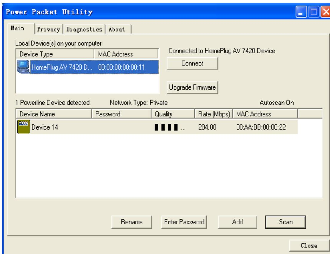
The lower panel displays all the HomePlugAV remote devices, which are discovered in the current logical network. The total number of remote devices connected in the same network is displayed above the remote device panel. **Network type (Public or Private)** depends on the network status of the local device. **Autoscan** shows whether the autoscan function is on. The following information is displayed for all the devices that appear in the lower panel.
