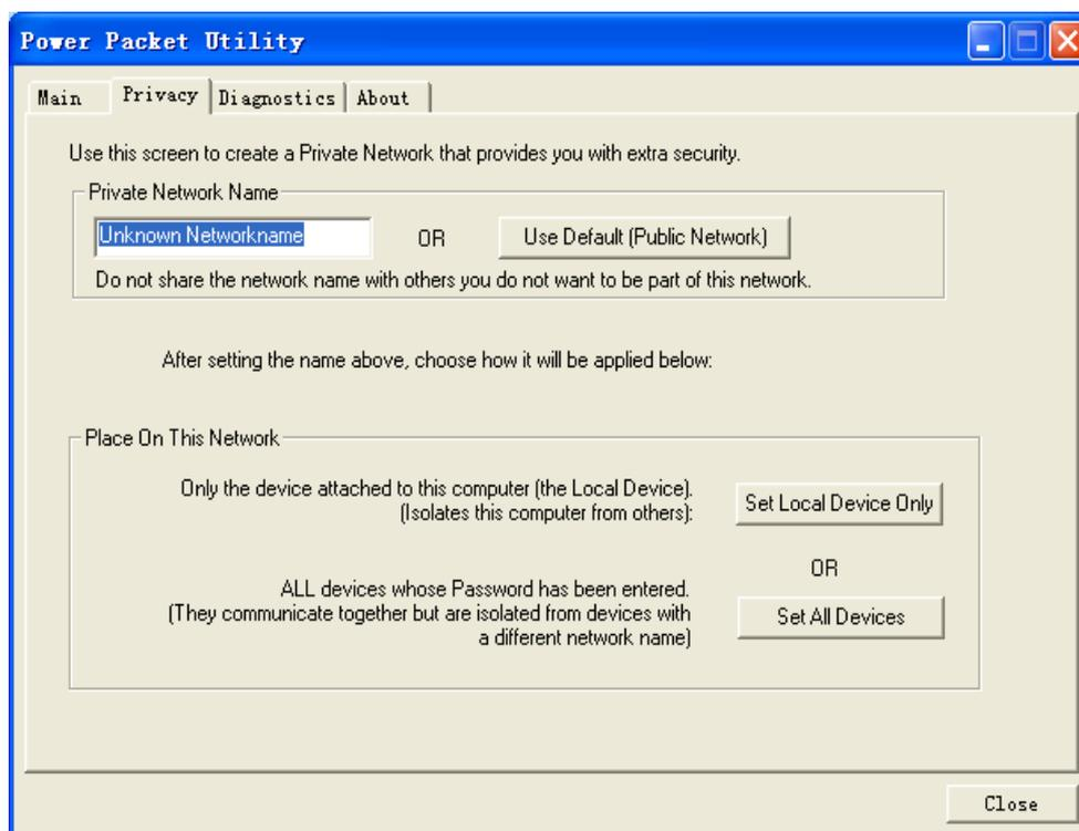
All HomePlugAV devices are loaded using a default logical network (network name), which is normally “**HomePlugAV**”. In the **Privacy** screen, you can modify a private network by changing the network names and the passwords of the devices.
