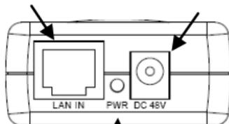
**PWR:** Power LED, a steady green light indicates that the PoE system has detected the PD or PoE Splitter and the power adapter is working properly.
