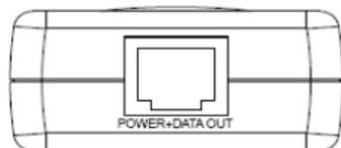
**POWER+DATA OUT:** Connect to the PD or PoE Splitter with a CAT5 UTP cable.
